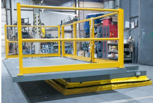
A remote 460/3/60 5 HP power unit and a deck installed 4 button control station operates the lift table raising and lowering and operates the sliding deck extension and retraction.
