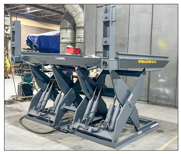
Two of the 3 photographs show the energy absorbing hinged deck stops in the raised locked position, the 3rd photograph (below) shows one of the deck stops in the raised position and the other in the lowered position. For assistance on any lift, lower or positioning application please contact the Pentalift Sales Department.
