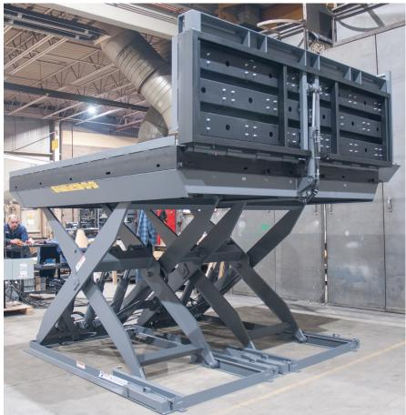
the guard rail installed control panel or the operators feet. The control panel operates the lift table up/down and the hinged tilt section of caster deck up/down. There is provision on the mounting plate for the overhead door controls to be installed.
