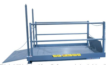
The Pentalift VCD dock lift, is surfaced mounted. This facilitates easy installation and lower installation costs. A pit is not required for installation of the lift. The low 5.25" lowered height makes pushing pallet jacks and hand dollies onto the lift easy.
