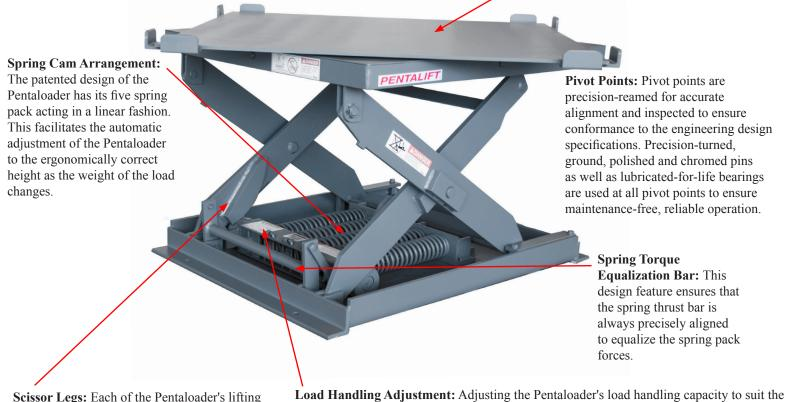
**Scissor Legs:** Each of the Pentaloader's lifting legs is precision cut from one piece of high tensile and high yield steel plate. The design profile of the legs has been engineered to provide both optimal support strength and maximum deck rigidity.
