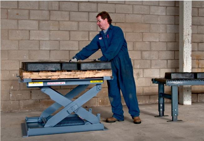
The Pentalift Pentaloader makes the palletizing job easier, safer and more efficient by automatically maintaining the height of the pallet at an proper ergonomic height. The top facilitates 360 degree rotation of the pallet to minimize reaching and stretching.
