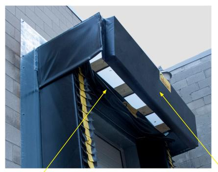
Designed to fit over existing dock seal head pads for retrofit applications. Rain water that would normally run into the facility is diverted to the sides of the trailer Oversized foam head curtain, reinforced with stays creates a positive seal on the top of the trailer roof.
