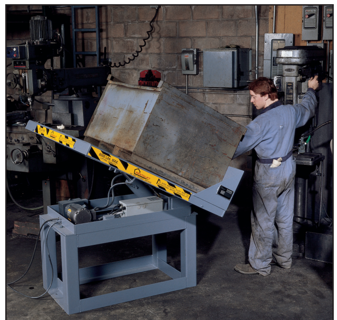
Pro-Series tilt table installed on a structural floor stand assembly.
