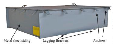
A pour in place dock leveler is provided with anchors and metal sheet siding to facilitate the concrete floor being poured around the dock leveler. The dock leveler is set into a foundation cut out, leveled and anchored in place, prior to the pouring of the concrete floor. When the concrete floor is poured the dock leveler is securely encased and installed. Field welding is eliminated. All the required welds are completed at the factory prior
