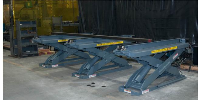
The lifts are shown in their location adjacent to the saw's main conveyor. The bundle of steel tubing to be cut is placed on top of the chain conveyors. It is prepared for loading onto the main saw conveyor. Due to the fact that the lifts are arranged adjacent to the main saw conveyor this preparation can be completed concurrently while the saw is cutting a bundle of steel.
