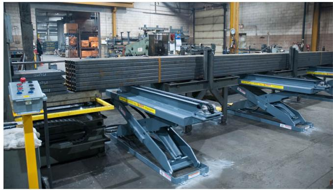
Once the bundle is lined up properly with the saw. The lift tables are lowered further to fully place the load on the conveyor and the sawing process commences.
