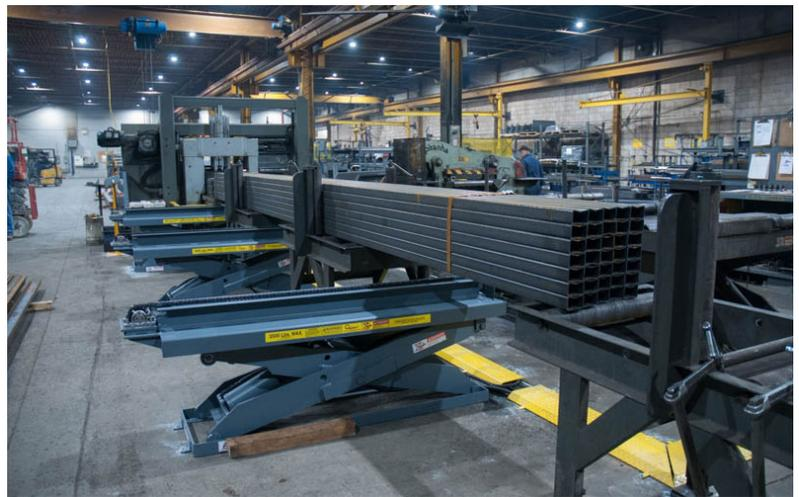
The lift tables are then positioned to receive the next bundle and repeat the process. This arrangement results in improved safety, productivity and efficiency by eliminating or significantly reducing saw dwell during loading. The saw can remain constantly cutting. This is a significant benefit in such an expensive machine center.
