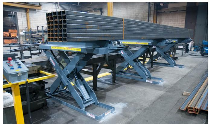
The lift tables are then lowered in synchronization to place the load on the conveyor. As the bundle approaches the conveyor the lift can be stopped and the side shifting chain conveyors can be shifted either direction as required to finely adjust the load to meet line up as required with the saws vice.
