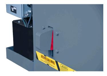
The color coded pawl indicates when the pawl system is engaged and it is okay to go under the fork truck maintenance lift. When red is visible on the locking pawl, do not go under the lift.
